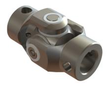
A customer was having a problem with a standard cross and needle bearing universal joint during the wash-down phase on the automation equipment of his food application. The needle bearing ioint would absorb the chemical solution used twice daily to clean and sterilize the equipment. Once the alloy bearings absorbed the chemical compounds, gumming would occur causing the joint to run tight, lock up and fail.
